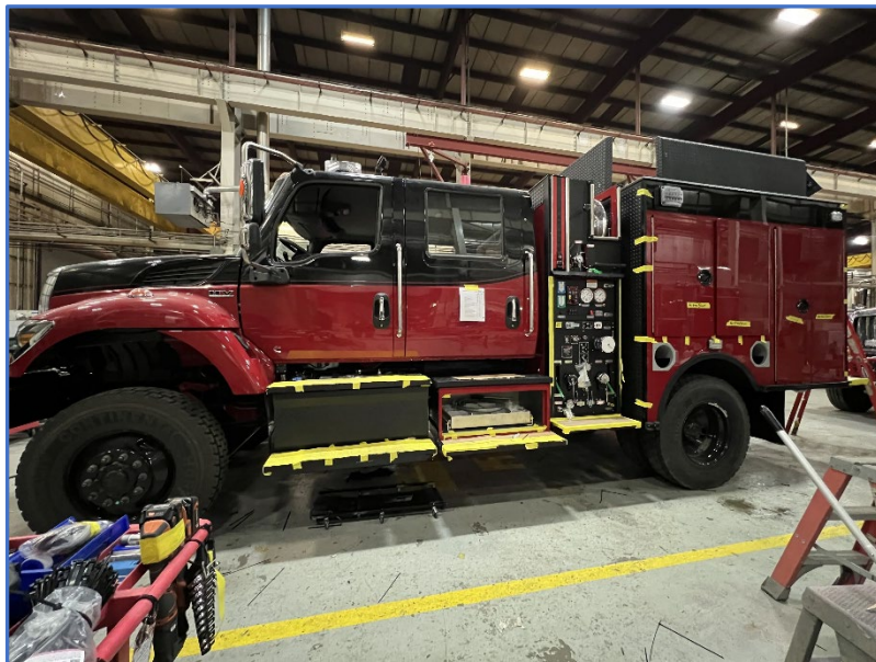
Type 3 engine under construction.
