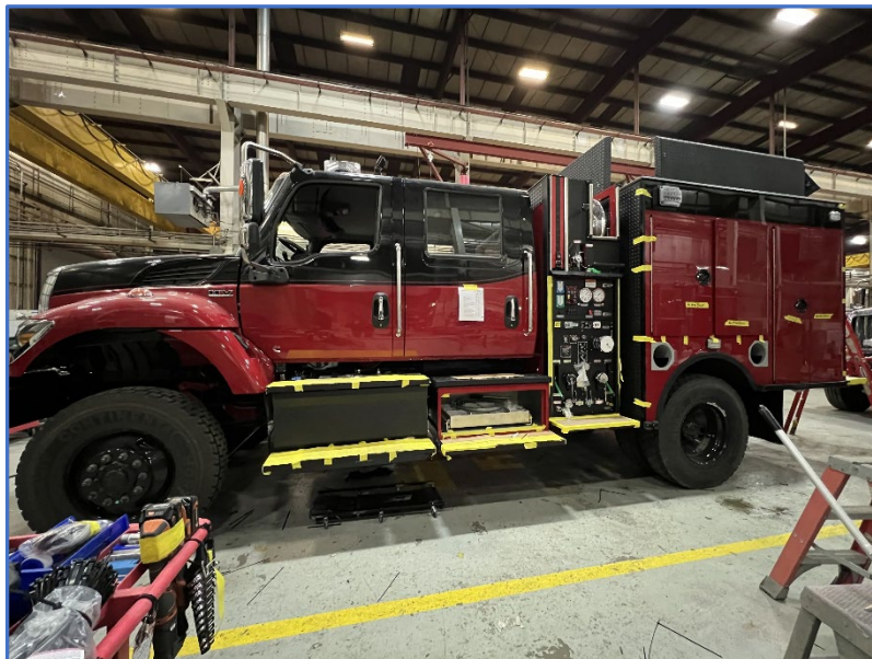
Type 3 engine under construction.
